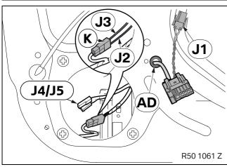
Insert the grommet **AD** into the hole.
