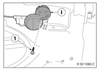
Install the tweeter I using the existing screw (1).
