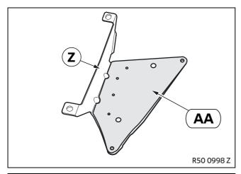
Place the drilling template **AA** on the holder **Z** and mark the holes.
