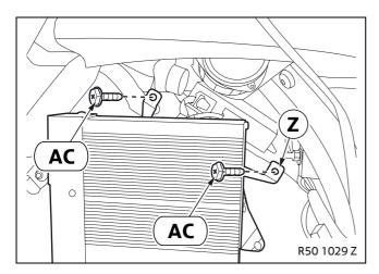
Secure the holder Z using speed nuts AC.
