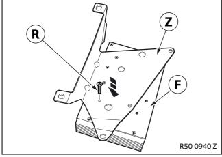
Secure the DPSM amplifier **F** to the holder **Z** using the screws **R**.
