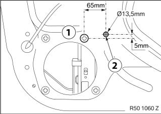
Mark the dimensions on the inside of the door (1) as follows and centrepunch at the drilling position (2).
