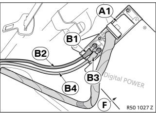
Connect branch A1 to the DPSM amplifier F.
