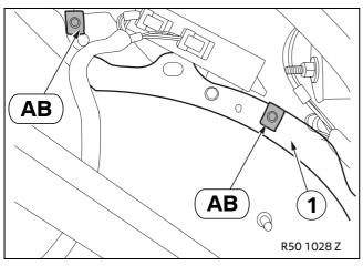
Fit the speed nuts **AB** to the holes on the body plate (1) in the boot at the rear right (behind the cover).
