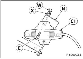
Secure the fuse **C1** to the mounting bracket **N** with fillister head screws **E**, toothed washers **X** and hexagonal nuts **W**.
