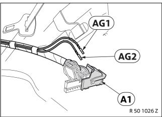
Route branch **A1** to the installation site of the DPSM amplifier **F**.
