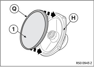
Remove the inside (1) of the seal **Q**.
