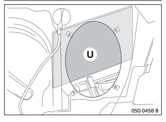
Affix the insulation mat  ${\bf U}$  to the side section behind the installation site for the rear speakers.
